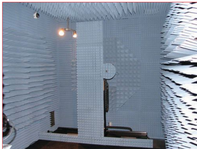
▲ Fig. 1 A near-field scanner moves an open-ended waveguide probe over a planar surface. Source: Concordia University in Montreal.
